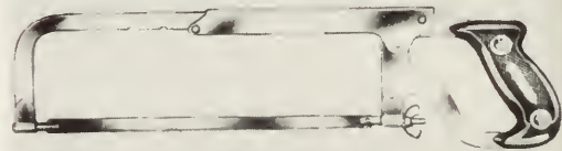
2-45. A hacksaw used to cut copper tubing and pipe. (Duro Metal Products Co.)
